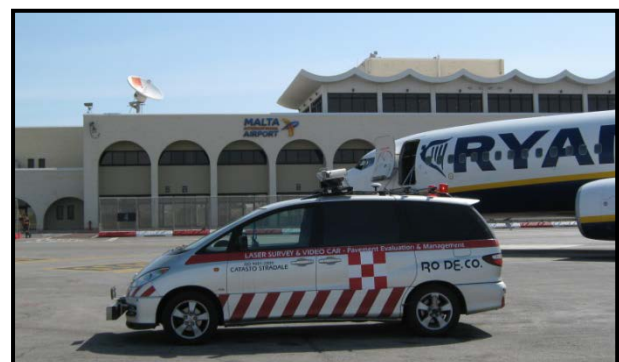
Fig.2 I.R.I. pavement roughness survey in the Malta Airport
